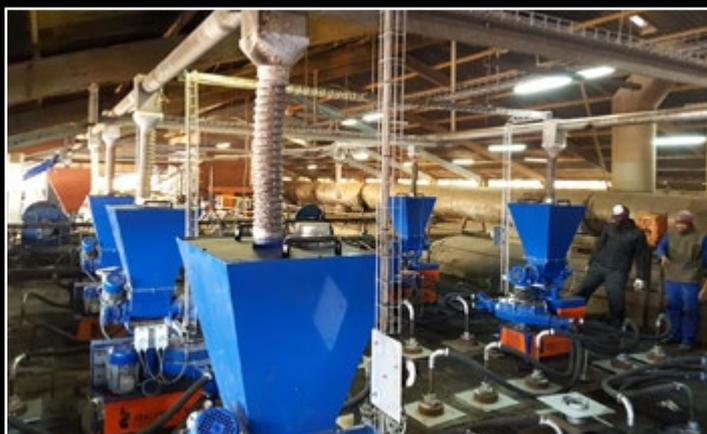
Bernini Impianti solid fuel kiln burners are designed for energy saving and improved combustion efficiency.
