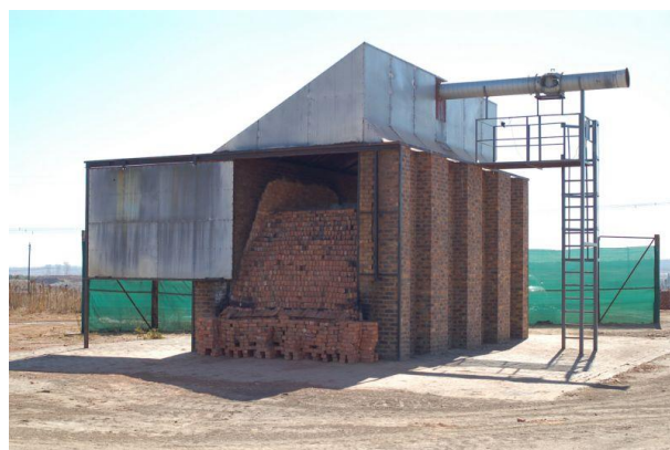
Figure 3: The model kiln provided real-world conditions for firing the clay brick, together with an accurate measurement system for measuring air emissions. The kiln was located far from general activities to ensure the minimum of contamination from other sources.
