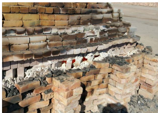
Figure 2: An open-air clamp kiln firing bricks
