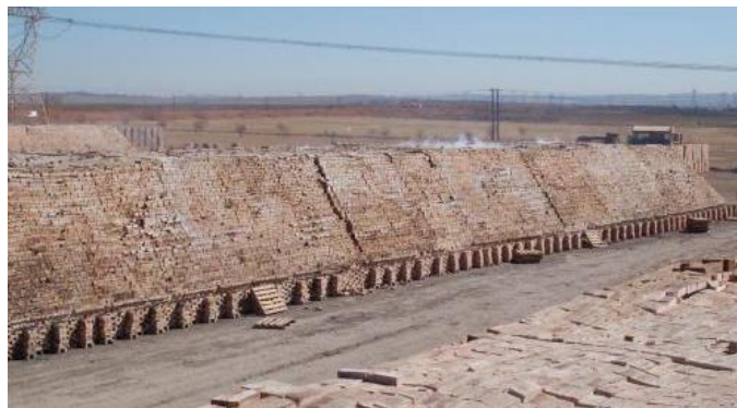
Figure 1: A full size clamp kiln. The model kilns takes a "slice" from the centre to duplicate firing conditions.
