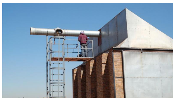
Figure 3: The model kiln provided real-world conditions for firing the clay brick, together with an accurate measurement system for measuring air emissions. The kiln was located far from general activities to ensure the minimum of contamination from other sources.
