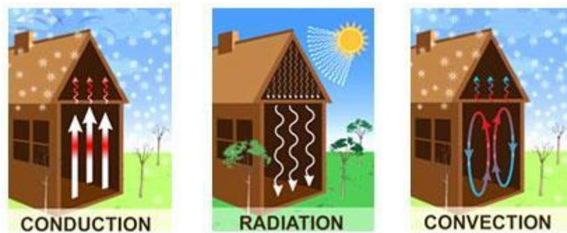
**CONDUCTION** is the molecule-to-molecule transfer of kinetic energy (one molecule becomes energized and, in turn, energizes adjacent molecules). A cast-iron skillet handle heats up because of conduction through the metal.
