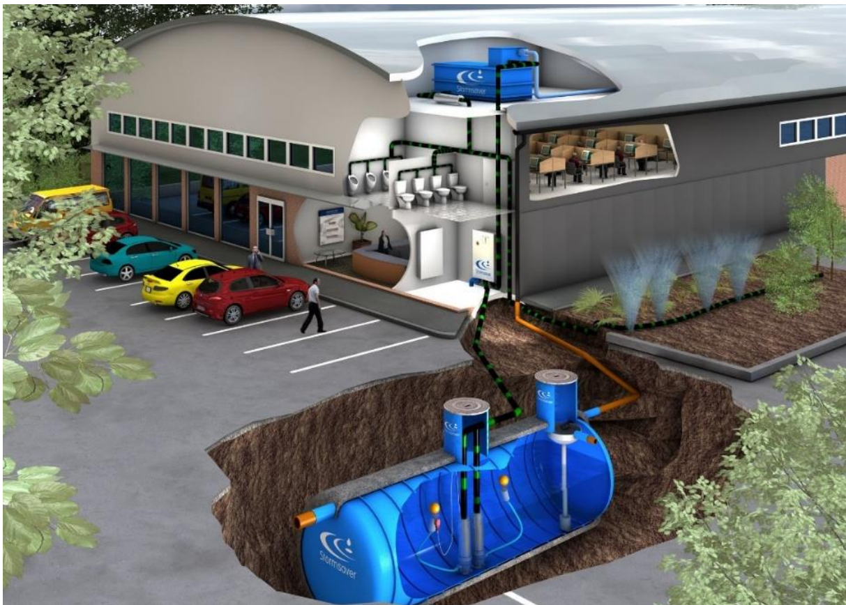
Figure 2 Underground Water Harvesting Tank Source: H2O Building Services (2018)
