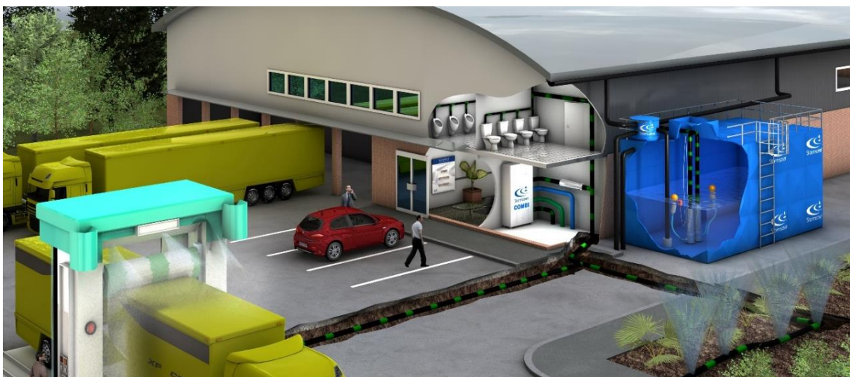
Figure 1 – Vertical Rainwater Collection Tanks Source: H2O Building Services (2018)
