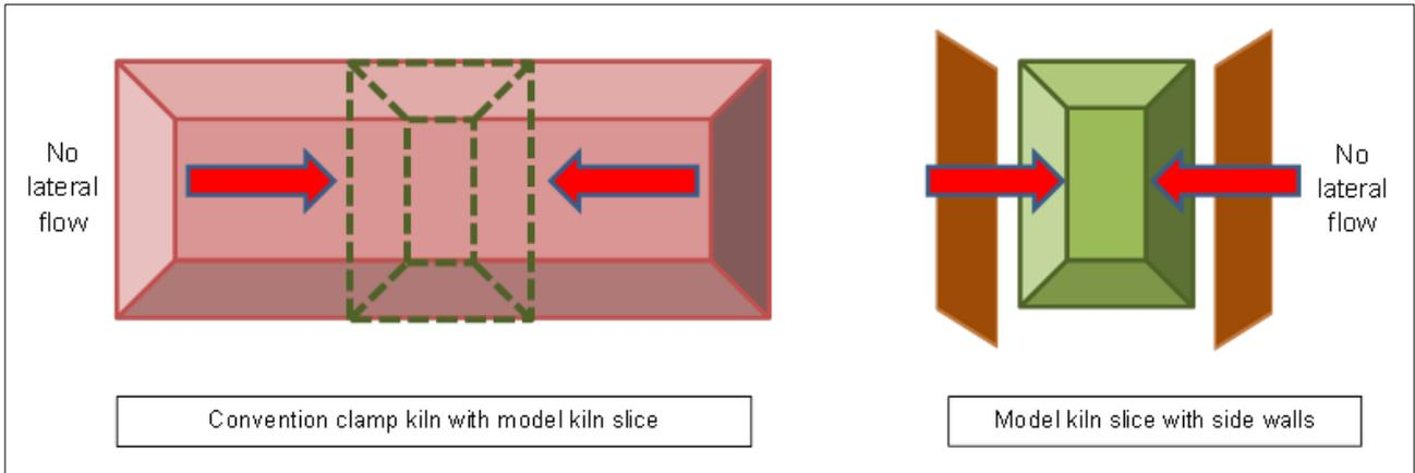
Figure 3: Illustration of air flow in a traditional South African clamp and the model kiln slice
