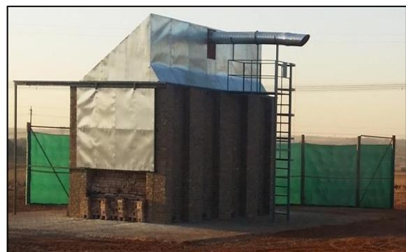
Figure 2: Model kiln showing horizontal stack and mesh windscreen
