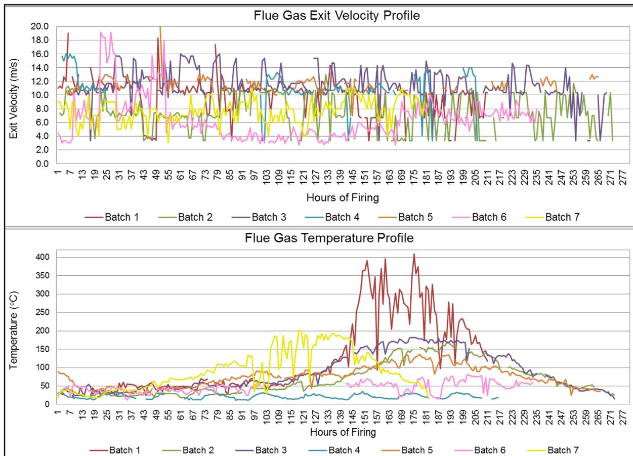
Figure 6: Flue gas velocity and temperature profile
