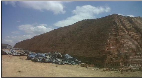
Figure 1: A typical kiln firing over seven million bricks in 21 days (Note: containment or extraction of emissions is not practicable)
