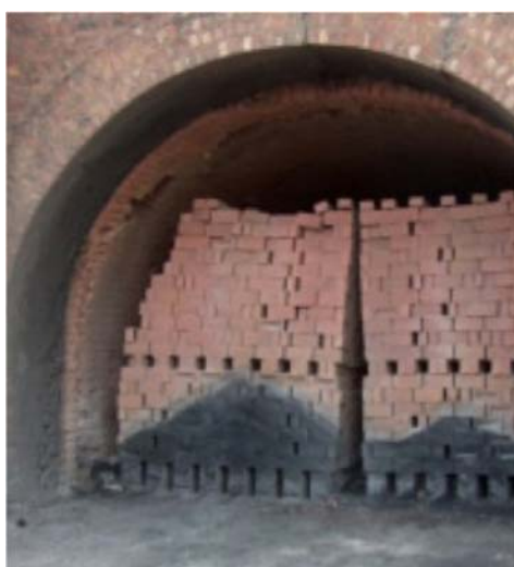
Figure 8: Transverse arch kiln (EcometrixAfrica, 2014).
