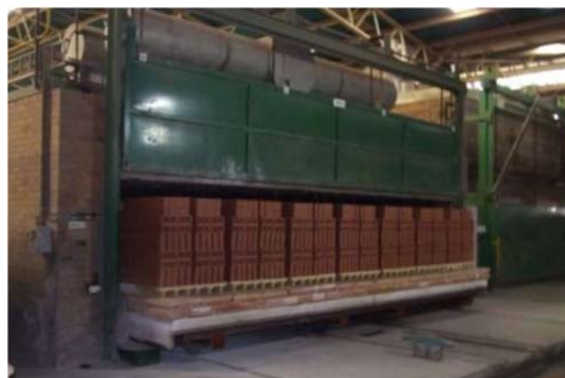
Figure 7: Dry bricks entering a gas fired tunnel kiln (Rice, 2012).
