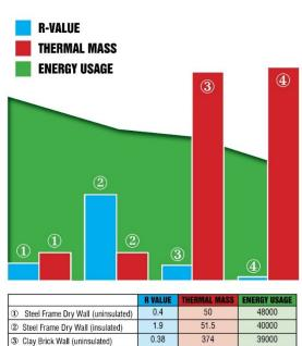
R-Value on its own has minimal impact on Energy Usage, until Thermal Mass is also taken into consideration.
