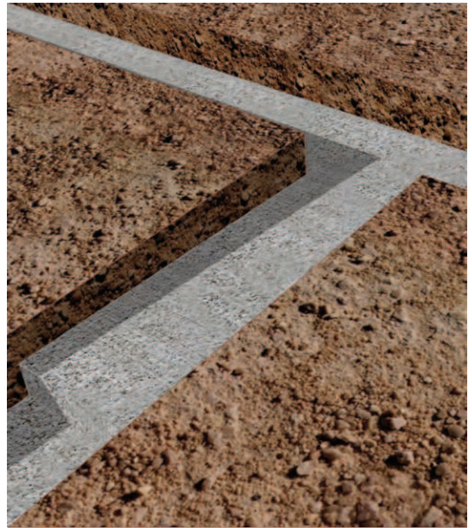
5.19 - Showing completed foundations with steps.
