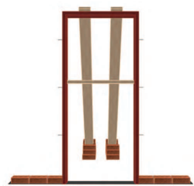
12.21 - Front view of the door frame. NOTE: The lugs and the centre strut (dwang) that is installed to prevent the frame from bulging in during building-in operations.
