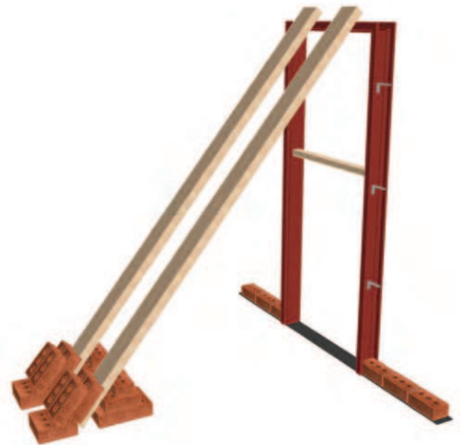
12.20 - Doorframe set upright in position on top of the D. P. C. As with window frames the door frame is secured in position with temporary supports.
