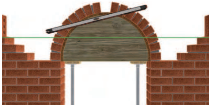
15.6 - Check the face of the arch with a level or a straight edge.
