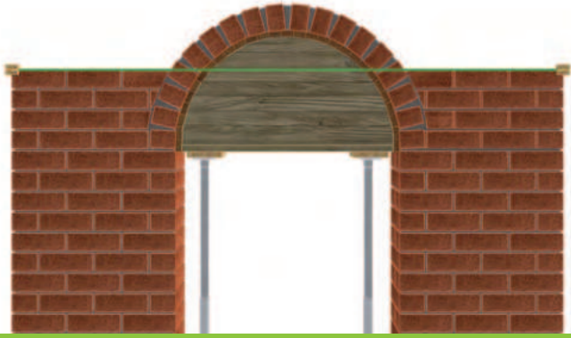
15.8 - Begin to build up the brickwork on either side of the arch. NOTE: The neat cutting in on the sides.
