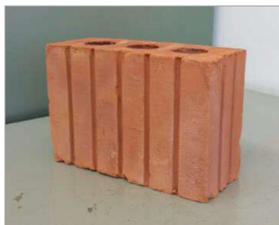
Figure 5: Narrow but double high for cavity walls. These bricks have been successfully used in cavity walling along the coastal belt
