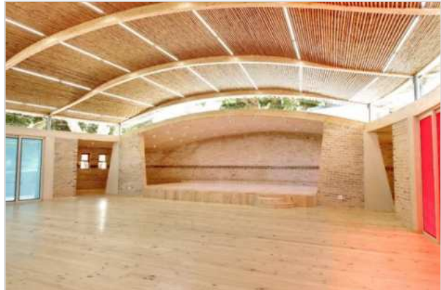
Figure 4: The dynamic double-curved clay brick walls, arching timber beams and slatted bamboo ceiling work together to provide a sustainable building with enhanced acoustics at the Constantia Waldorf School. Photo courtesy of Corobrik.
